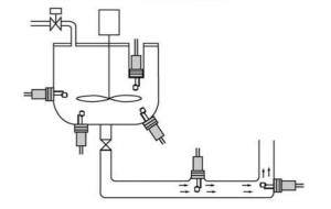
Bi-directionally oscillatory detector head driven by Piezoelectric acceleration allows any direction of flow against the head.
